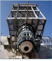
Figure 10: A solid propellant rocket motor on a test stand. (Avio SpA)
