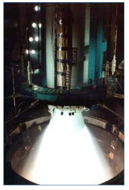
Figure 11: A full scale solid rocket engine being tested at simulated high altitude. (AEDC)
