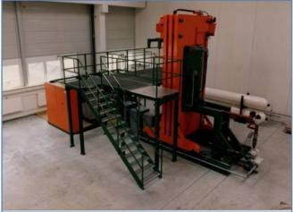
Figure 6: Left: A laboratory sized isostatic press. (ESPI) Right: A laboratory sized hot isostatic press. (Abra Fluid AG)
