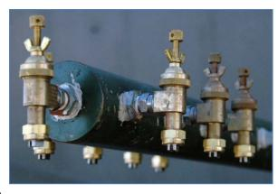
Figure 4: A Modular Aerial Spray System, used for pesticide application, can use a setting called ultra-low volume and specialized spray boom nozzles such as those shown here to spread one half to an ounce of chemical over an acre. (U.S. Air Force)
