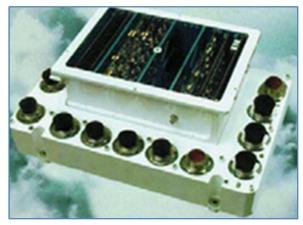
Figure 6: Digital signal processor with the lid removed. The size is 5 cm to 7.5 cm on each side. (MTCR Equipment, Software and Technology Annex Handbook, Third Edition (May 2005))
