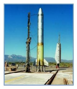
Figure 3: Minimal launch pad with a gantry and connections to a complete rocket system. (MTCR Equipment, Software and Technology Annex Handbook, Third Edition (May 2005))
