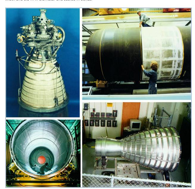
Figure 9: Top left: An engine with a large, regeneratively cooled nozzle. (MTCR Equipment, Software and Technology Handbook, Third edition (May 2005)) Bottom left: Installation of insulation inside a filament wound rocket motor case. (Thiokol Corp.) Top right: A rocket motor case under inspection after application of the thermal insulation. (Fiat Avio) Bottom right: Side view of a regeneratively cooled nozzle. (Boeing)
