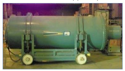
Figure 15: A 2.3MeV flash X-ray unit used for inspecting solid rocket motors. (MTCR Equipment, Software and Technology Annex Handbook, Third Edition (May 2005))
