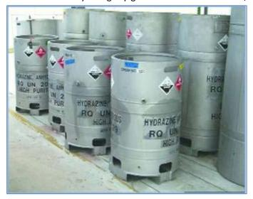
Figure 9: 34-gallon anhydrous hydrazine shipping containers made of 300-series stainless steel. (MTCR Equipment, Software and Technology Annex Handbook, Third Edition (May 2005))
