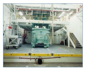
Figure 4: A 420-gallon propellant mixing bowl. (ATK)
