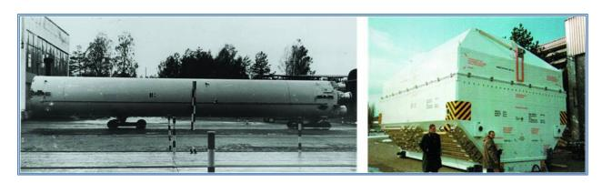
Figure 2 *Left:* The first stage of a liquid-fueled ICBM. *Right:* A shipping container for a liquid-fueled upper stage. (MTCR Equipment, Software and Technology Handbook, Third edition (May 2005))
