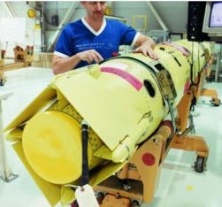
Figure 10: Left: A Space Launch Vehicle on an assembly jig. (Korea Times) Right: Modular jig supporting a cruise missile in final assembly.
