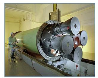
Figure 4: A finished motor being X-rayed to ensure that the propellant grain is homogeneous, bonded to the case, and free from cracks and other imperfections. (ATK)
