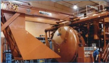
Figure 8: Left: A large scale custom CVD furnace which inductively heats graphite to temperatures in the 2800 °C range. (CVI) Right: A large CVD furnace. (Seco Warick)
