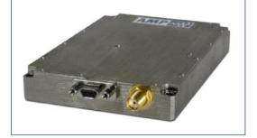
Figure 11: Some telemetry transmitters are designed to withstand harsh operating environments requiring compact and rugged package. (AMP)
