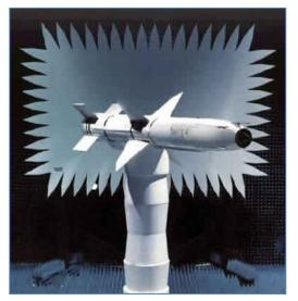
Figure 5: A target missile in the Bistatic Anechoic Chamber (BAC) RCS measurement compact range. (U.S. Navy)
