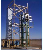
Figure 9: A vertical test stand designed for testing liquid propulsion rocket engines. (Interorbital
