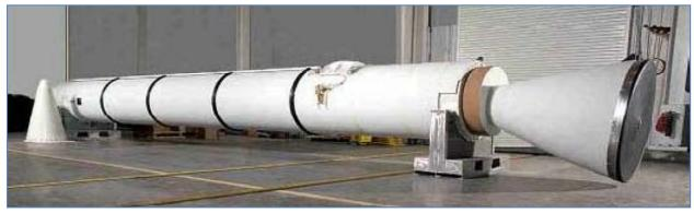
Figure 8: A rocket motor with large fixed nozzle. The motor is used on a launch vehicle. (ATK)
