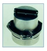
Figure 10: A dynamically tuned gyro (DTG). (The Charles Stark Draper Laboratories, Inc.)
