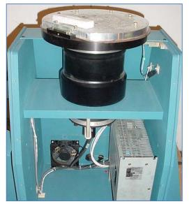
Figure 21: A typical rate table used for tuning gyros. (Ideal Aerosmith, Inc)
