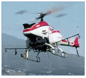
Figure 5: A rotary-wing UAV designed with chemical tanks and spraybars for agricultural purposes. (Yamaha)
