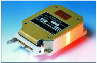
Figure 12: *Top left:* three exposed ring laser gyros without their associated electronics. (Honeywell) *Top right:* a fiber optic gyro with its top removed. (Honeywell) *Bottom:* a fiber optic, rate sensing gyro. It is 2 cm x 6.5 cm x 8 cm. (LITEF)
