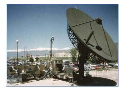
Figure 13: A large SATCOM military antenna designed for major command posts and mobile command posts, and suitable for communications with UAVs. (General Dynamics)
