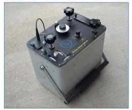
Figure 9: This automated gravity meter is one of the most precise, rugged and lightweight gravity meters. Under normal conditions, it can be leveled for mGal readings within 30 seconds, and has a drift rate of less than 0.5 mGals per month when mature. (ZLS Corporation)
