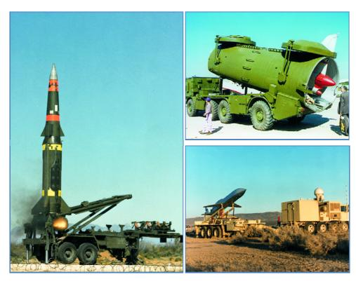
Figure 7: *Left*: an erector launcher detached from its prime mover. (MTCR Equipment, Software and Technology Annex Handbook, Third Edition (May 2005)). *Top right*: a transporter erector launcher for a large, Category II cruise missile. (MTCR Equipment, Software and Technology Annex Handbook, Third Edition (May 2005)). *Bottom right*: Erector launcher for a rocket-assisted UAV and its associated command-and control van. (Teledyne Ryan Aeronautical)
