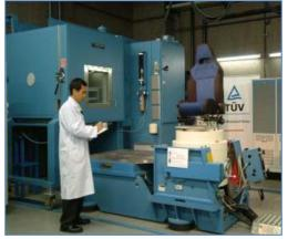
Figure 13: A vibration and environmental test apparatus configuration. (TUV Rheinland)
