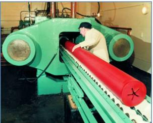
Figure 5: A finished motor being X-rayed to ensure that the propellant grain is homogeneous, bonded to the case, and free from cracks and other imperfections. (ATK)
