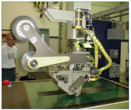
Figure 3: An automated tape-laying machine head. (Automated Dynamics)
