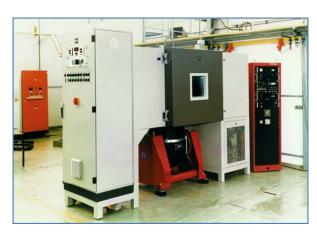
Figure 12: A controlled environmental chamber with vibration capability. (RMS Dynamic Test Systems)
