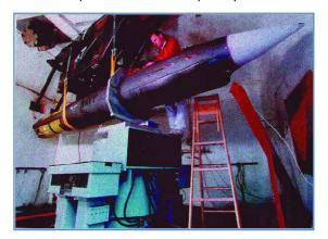
Figure 2: A thruster being prepared to vibration-test a missile. (Unholtz-Dickie)
