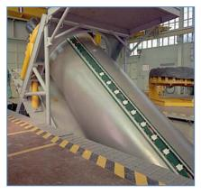
Figure 3: Solid propellant in liquid form is poured into rocket casings and cast into the required shape. The casting is moved by a hydraulic mount to remove bubbles or other defects. (ATK)
