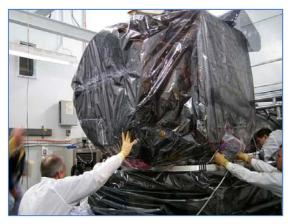
Figure 1: Vibration testing of a laser altimeter system. (NASA)
