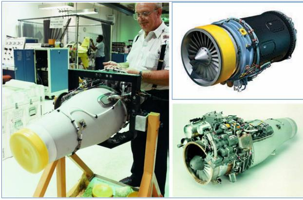
Figure 1: Left: A small turbofan engine for a cruise missile on its checkout stand. (MTCR Equipment, Software, and Technology Annex Handbook, Third Edition (May 2005)) Top right: A turbofan used to power a HALE UAV. (Rolls Royce Group, plc) Bottom right: A small turbofan engine for a cruise missile. (Williams International)
