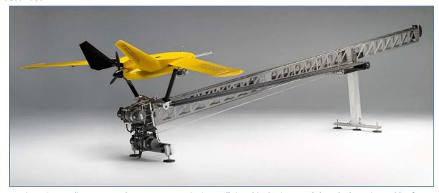
Figure 3: A medium-range endurance UAV. Despite its small size, this elastic catapult-launched UAV is capable of carrying a 1 kg payload (IR and digital cameras) to a range of 400 km. (Aerovision Vehiculos Aereos, SL)
