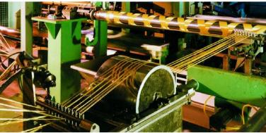
Figure 5: Left: A prepreg machine constructed by the Composite Materials Group for the production of prepreg materials using fibers and resins. (Katholieke Universiteit Leuven) Right: A machine adding resin to seven lines of roving. (Hunting Engineering, Ltd.)
