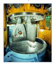
Figure 5: Solid propellant being mixed in a 600-gallon vertical planetary mixer. (Thiokol Corp.)
