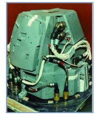
Figure 1: The main body of a cruise missile's integrated flight instrumentation system. (Litton **Guidance and Control Systems**)
