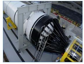
Figure 8: The load measurement system on the test stand of a solid rocket motor. (ATK)
