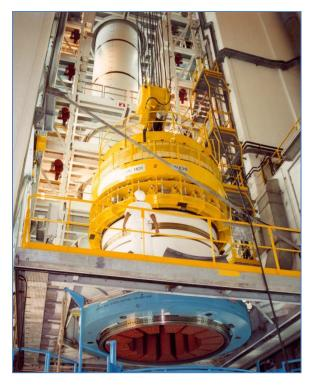
Figure 1: Integration of a satellite launch vehicle booster with the solid propellant rocket motor stage (above). (European Space Agency)
