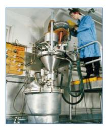
Figure 2: Slurry cast double-base mixing equipment for a small motor. (British Aerospace Limited)
