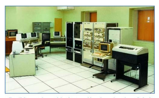
Figure 15: Representative ground-site telemetry receiving and processing equipment. (In-Snec)
