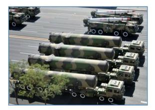
Figure 4: Above: Eight axle and four axle TELs carrying intercontinental ballistic missiles (ICBMs; foreground) and intermediate range ballistic missiles (IRBMs). (Via Chinese Internet)
