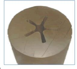
Figure 8: A sample of double-base rocket motor propellant. (Bayern-Chemie GmbH)
