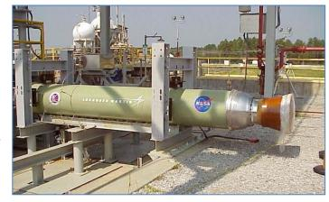
Figure 14: A hybrid sounding rocket motor. (NASA)
