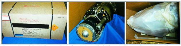
Figure 2: Left: A turbojet shipping crate showing the explosive warning labels required because of the starting cartridge. (Teledyne Ryan Aeronautical) Center: A small turbofan engine wrapped in plastic inside its shipping crate. (Teledyne Ryan Aeronautical) Right: A small turbojet engine being prepared for shipment. (Teledyne Ryan Aeronautical)
