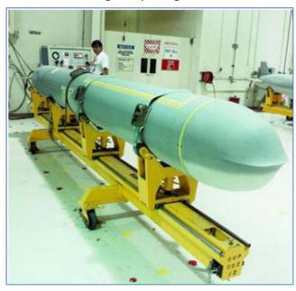
Figure 7: An operational cruise missile on its checkout stand, showing its nose cone modified to lower radar returns and enhance aerodynamic performance. (MTCR Equipment, Software and Technology Handbook, Third edition (May 2005))
