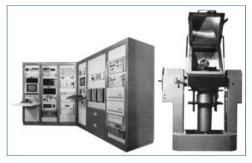
Figure 22: A two axis rate integrating gyro test station utilizing a motion simulator / rate table. (Contraves, Inc)
