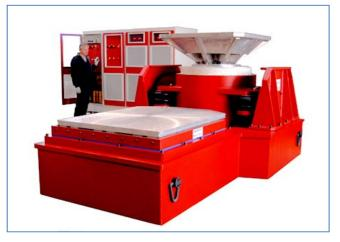
Figure 4: An example of a thruster with slip table. (Kingdom Pty Ltd)
