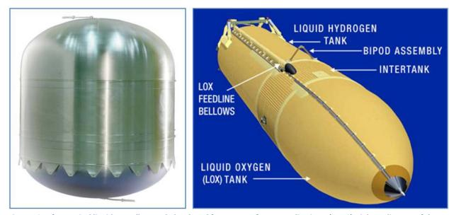
Figure 16 *Left:* A typical liquid propellant tank developed for a range of space applications. (EADS) *Right:* A diagram of the external tank used by a space vehicle launch engine, showing the separated oxidizer and fuel tanks. (NASA)
