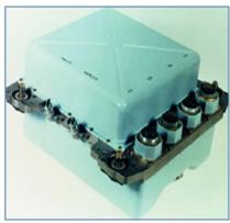
Figure 3: A radiation-hardened electronics assembly with liquid cooling. (The Charles Stark Draper Laboratory, Inc.)
