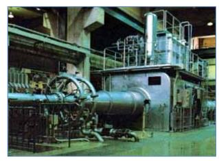
Figure 5: A hypersonic wind tunnel capable of equaling Mach 5 to test flight conditions for launch vehicles. (Mitsubishi Heavy Industries, Ltd)
