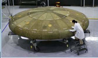
Figure 5: Left: A beryllium-copper heat sink. (National Atomic Museum) Right: A prototype heat shield for use on vehicles during re-entry from lunar and low-Earth orbit missions. (Boeing)
