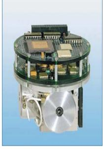
Figure 15: An Inertial Measurement Unit (IMU) utilizes inertial fiber optic gyros (FOGs) and micro-machined accelerometers and is used in space stabilization, missile guidance, UAV guidance and flight control. (Northrop Grumman)
